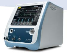
The SLE6000 is a high-specification, compact infant ventilator that offers a range of conventional modes with additional options for volume targeted ventilation (VTV) non-invasive ventilation (NIV), high frequency oscillation ventilation (HFOV) and high flow oxygen therapy.
